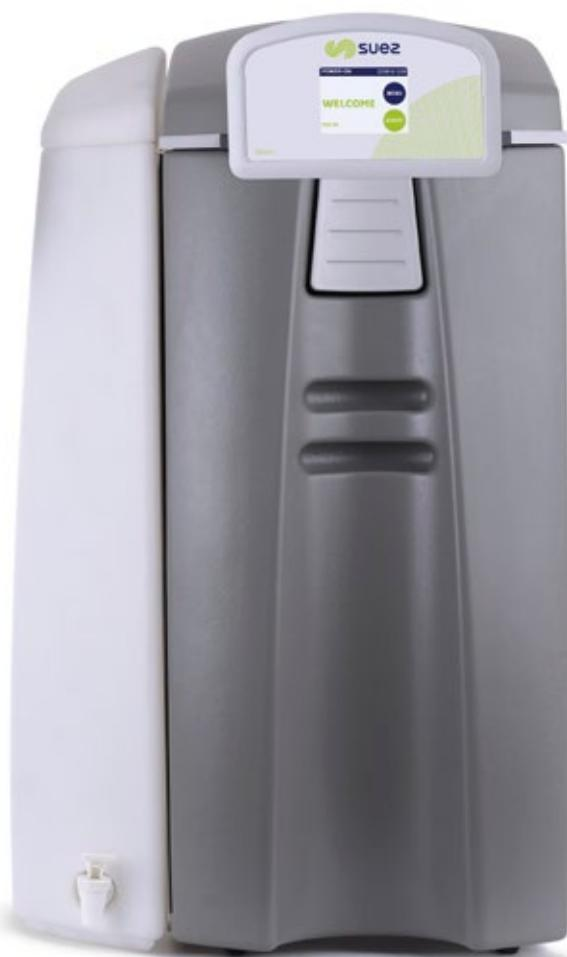
The Select edi 60 is a compact unit ideal for laboratory use delivering a constant supply of >5MΩ.cm pure water for laboratory tasks using activated carbon pre-treatment, double pass reverse osmosis, carbon dioxide membrane degassing and electro-deionisation technology.
