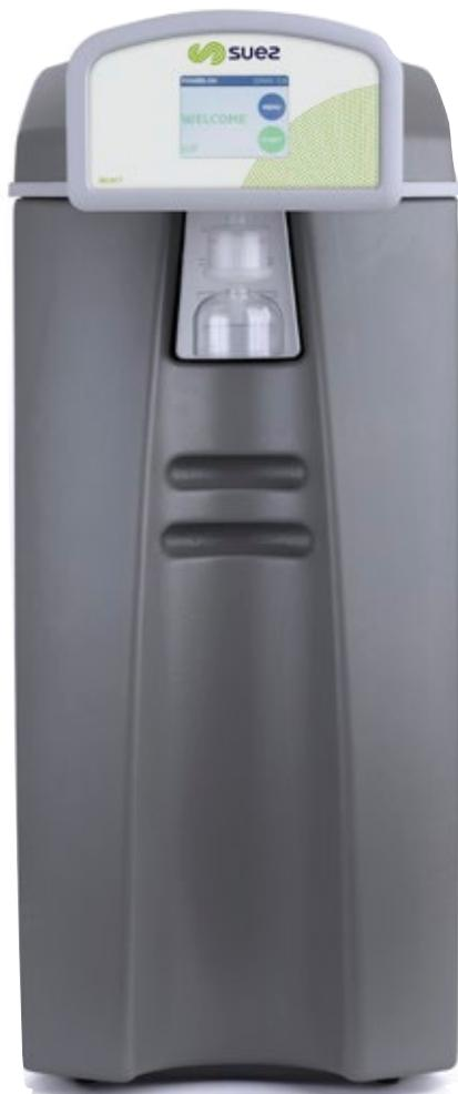
The Select Neptune Ultimate provides a high flow of guaranteed 18.2MΩcm ultrapure water for analytical and life science laboratory applications.
